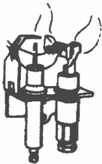
Fig. 2: Pilot Burner Flame
